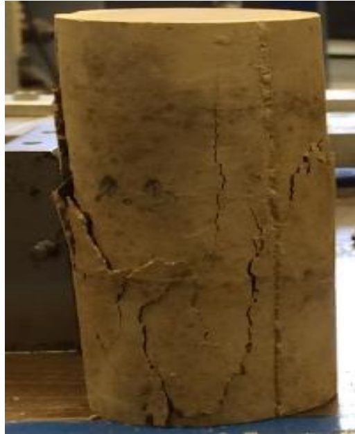
Figure 3-14: Typical shear failure of the specimen in compression
