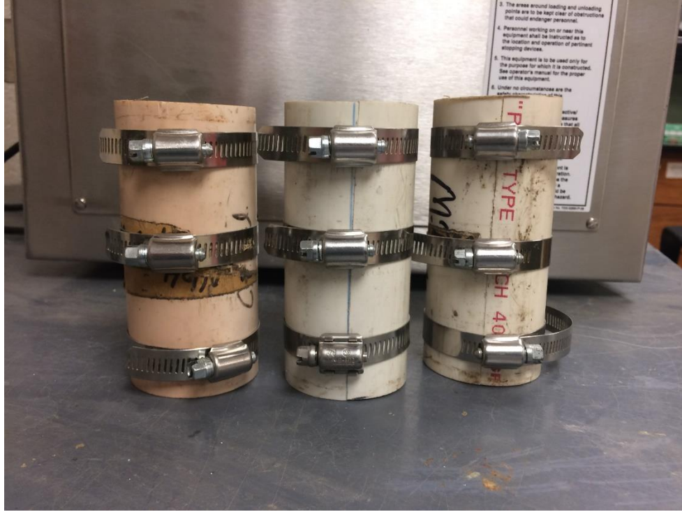
Figure 3-7: Restrained of the mold using stainless hose clamp
