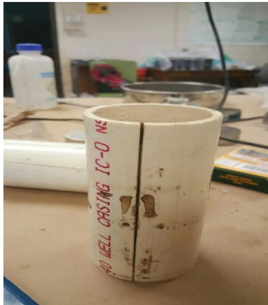
Figure 3-6: Plastic mold with vertical slit
