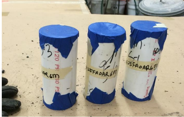
Figure 3-8: Sealed sample for before curing
